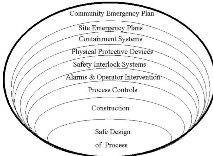
Figure 1 Defence-In-Depth Approach to Safe Operation of a Facility
