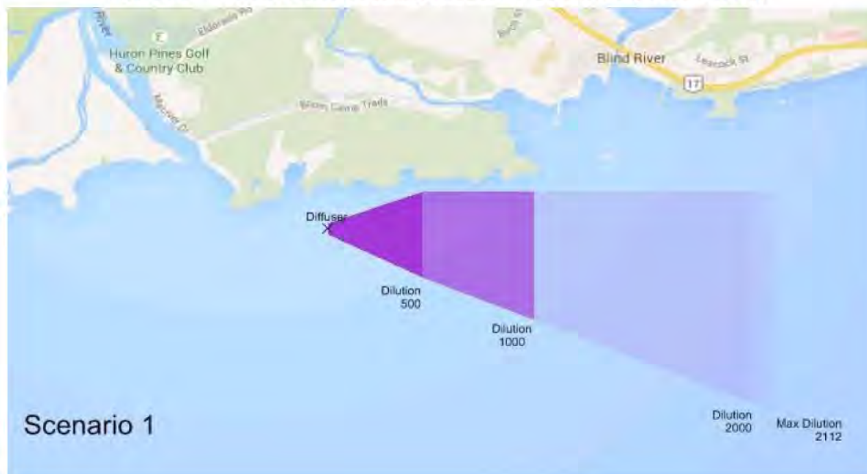
Figure 3.3 CORMIX Plume Modelling Results for 'Scenario 1' (Arcadis 2015a)
