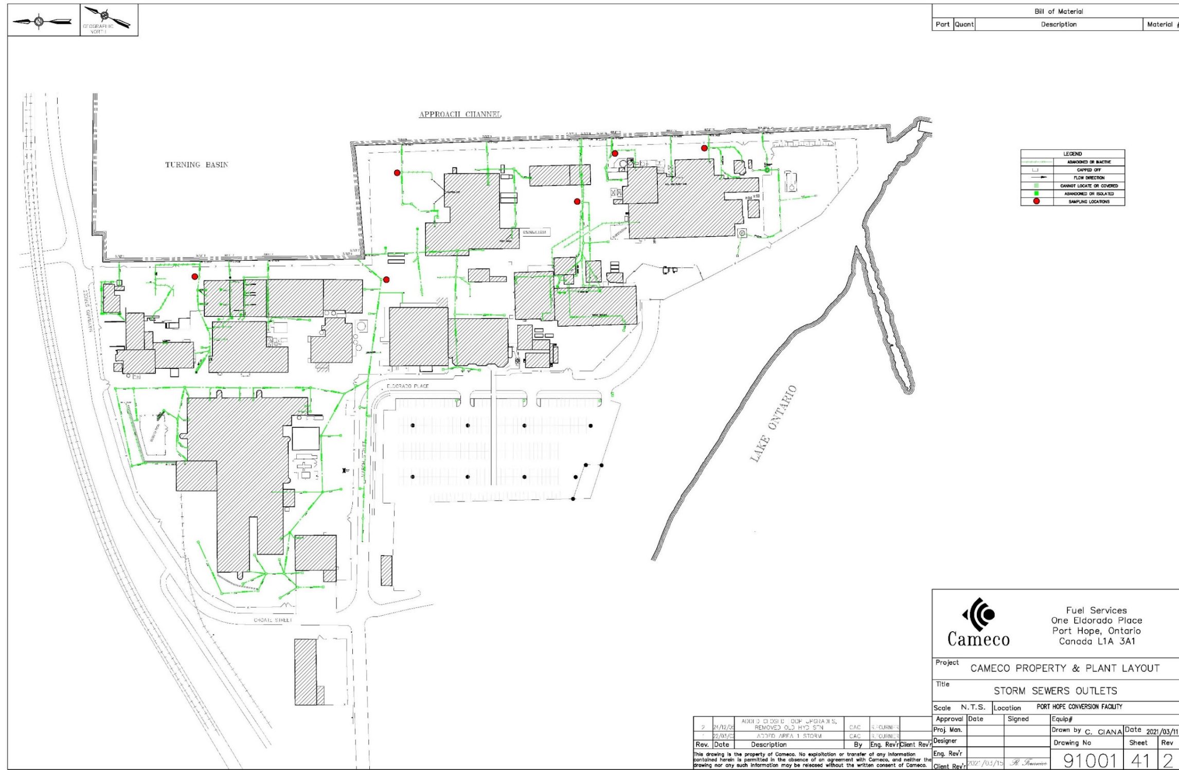
Figure 36: Storm Sewer Outlets
