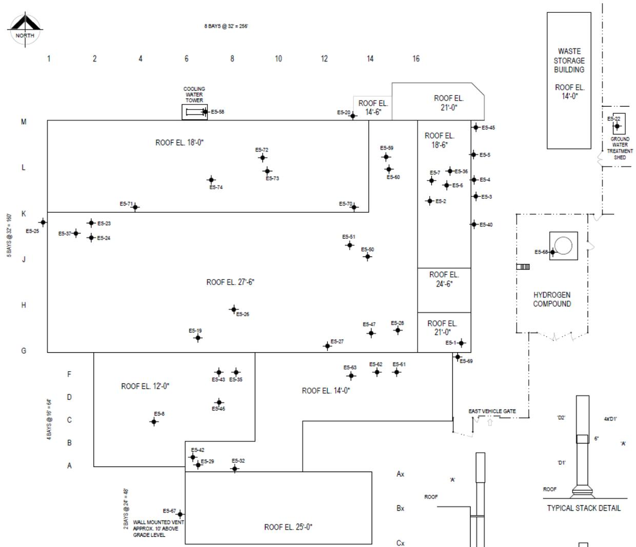
Figure 2 CFM Liquid Sampling Points
