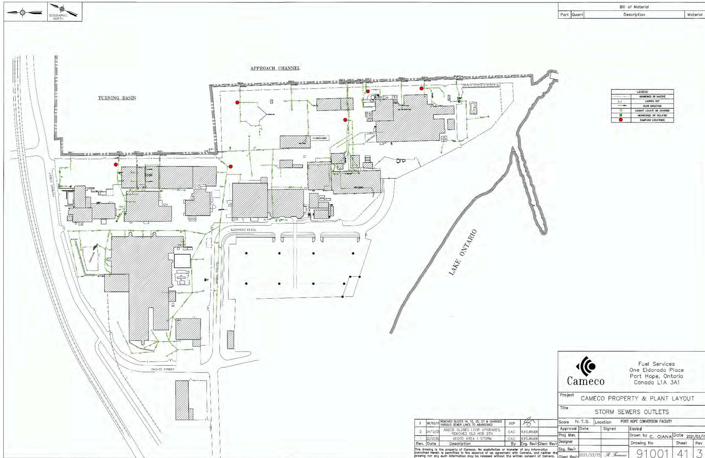
Figure 30: Storm Sewer Outlets
